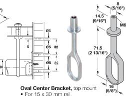
mounts with M6 screw Material: zinc die-cast
